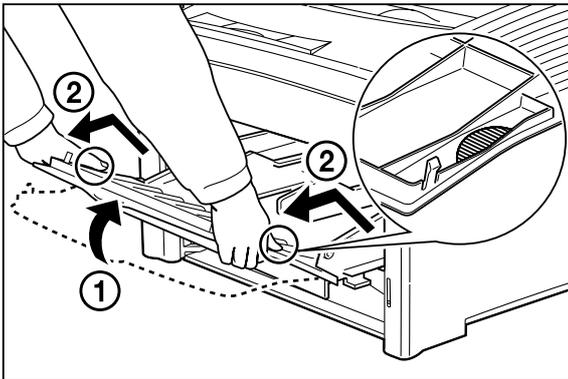
11. Hold the EP cartridge as shown in the illustration and pull it out slowly.
