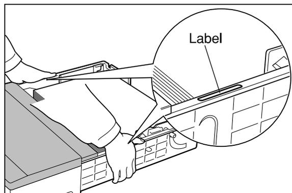
10. Insert the cassette fully into the printer at the both hands. Make sure that the cassette is properly seated.
