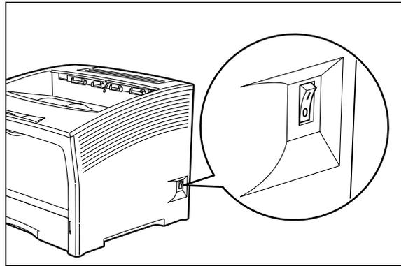
2. Then disconnect the power cord from the AC outlet and the printer.
