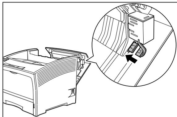
8. Gently lower the HCS unit onto the printer while inserting the metal fittings of the HCS unit into the metal fittings on the printer.
