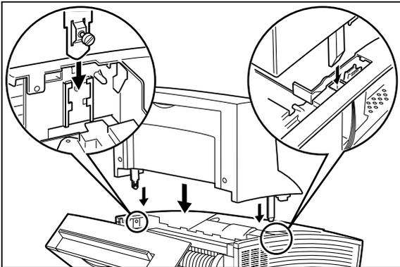
9. Secure the HCS unit to the printer with the supplied screw.
