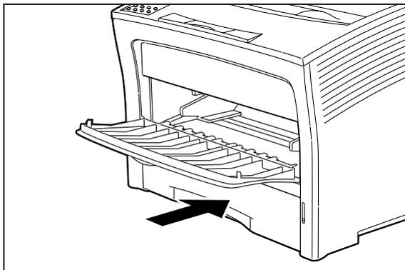
If the optional paper feeder is installed, replace the paper cassette removed earlier.
