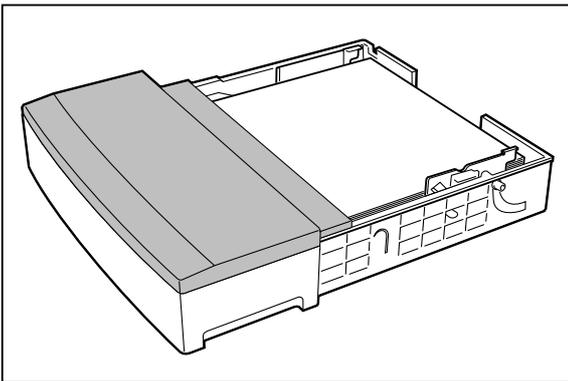
11. Insert the cassettes all the way into the printer. Make sure the cassette is properly seated.
