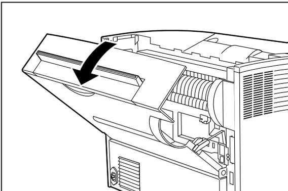
5. Remove the cover at the location where the HCS will be installed.
