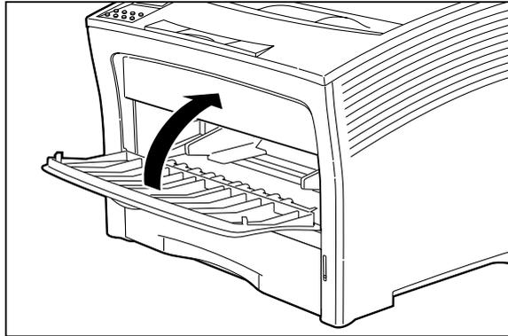
7. Gently lift the cassette up and remove it from the printer.
