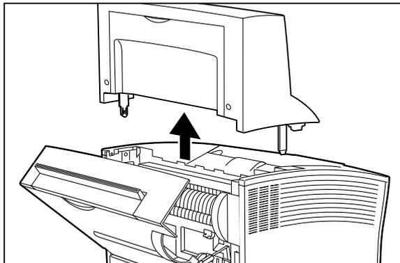
7. Re-install the cover at the location where the HCS was located.
