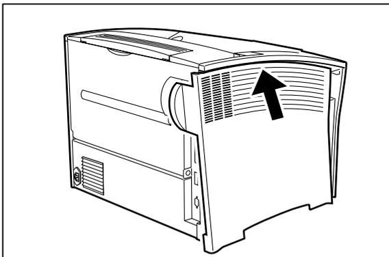
2. Align the projecting parts on the cover with the holes on the lower left side of the printer.
