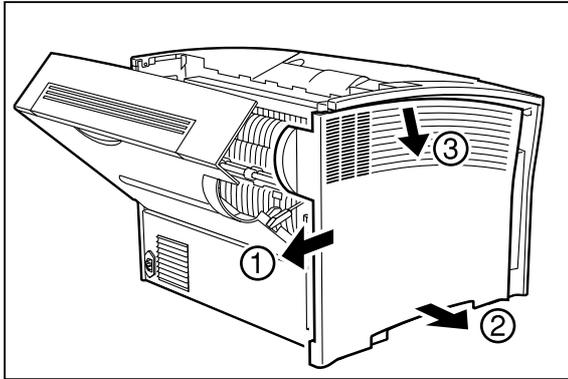
4. While holding the orange tabs on the duplex printing unit, pull the unit towards you to remove it from the printer.
