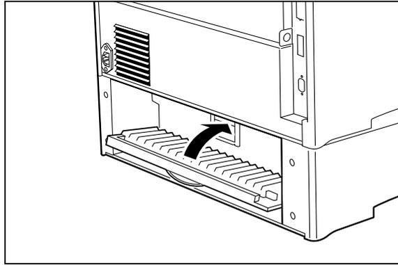
7. Pull on the recessed area to open the top rear cover, as shown.
