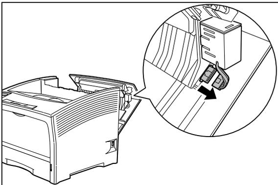
9. Press the claw on the attachment and remove the attachment from the rear cover.
