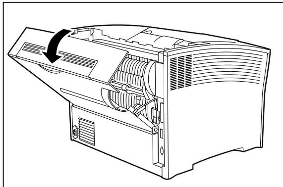
3. Remove the cover on the left side of the printer.
