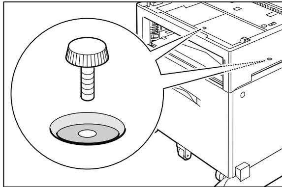
8. Lower the printer onto the HCF unit or the paper feeder.
