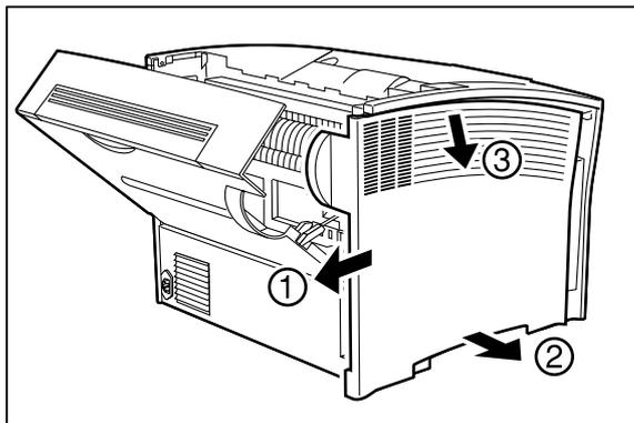
4. While holding the orange tabs on the duplex printing unit, insert the two pins on the lower part of the duplex printing unit into the openings on the printer.
