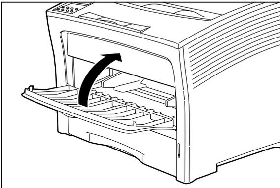
5. Gently lift the cassette up and remove it from the printer.
