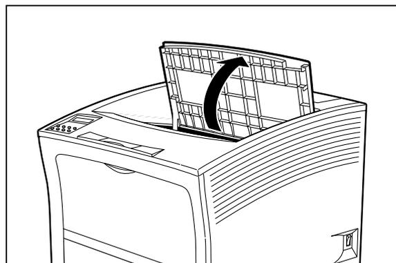
2. Pull on the recessed area to open the top rear cover, as shown.
