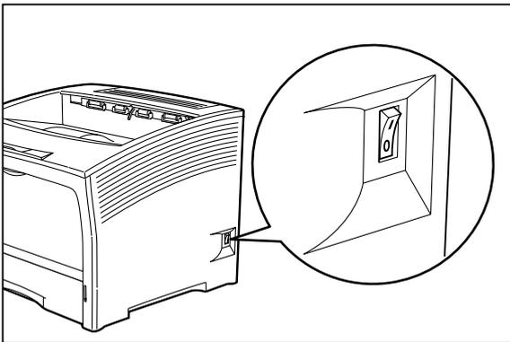
5. Then disconnect the power cord from the AC outlet and the printer.
