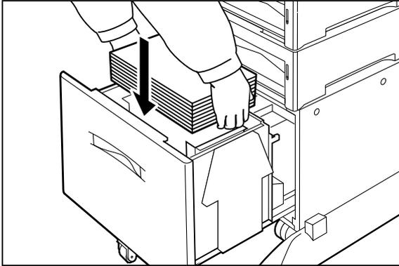
11. Insert the cassette completely the printer. Make sure the cassette is properly seated.
