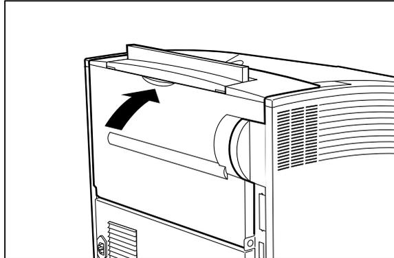
11. Use coins or similar objects to insert into the space below the HCS cover (located on the top rear side of the printer) and gently push them down, then remove the cover.
