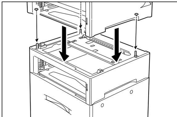
9. Insert the two supplied screws into the holes on the inside of the cassette feeder of the printer to secure the paper feeder.
