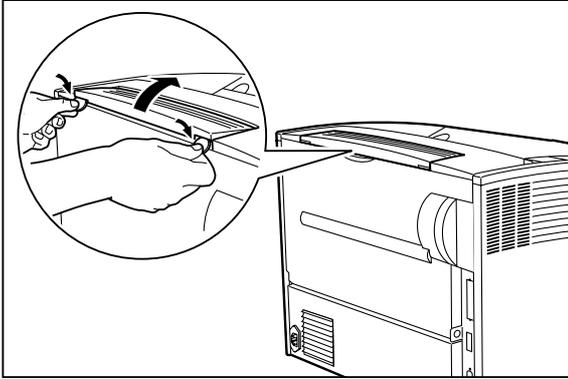
3. In place of the cover removed, install the cover supplied with the HCS unit.
