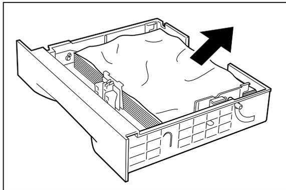
6. Check the far end of the cassette feeder, and remove any jammed paper.
