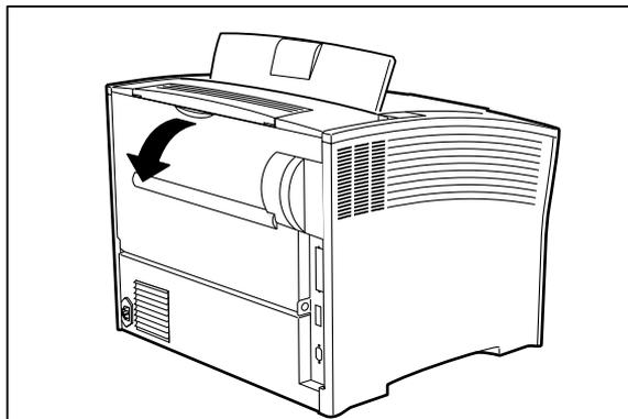
8. Open the lever on the left side of the fuser and remove any jammed paper.
