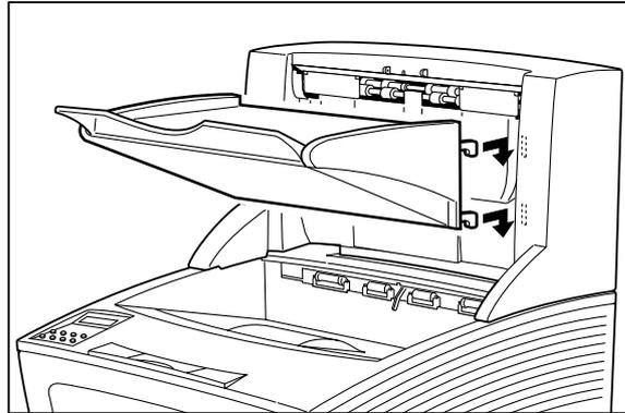
12. Insert the projecting part of the paper stopper into the hole at the upper part of the paper exist slot.
