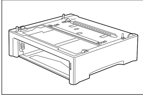
2. While aligning the 3 stubs on the 2nd feeder with the holes on the bottom of the 1st feeder, stack the 1st paper feeder onto the 2nd paper feeder.
