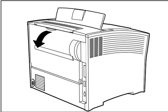
3. Check and carefully pull out any jammed paper.
