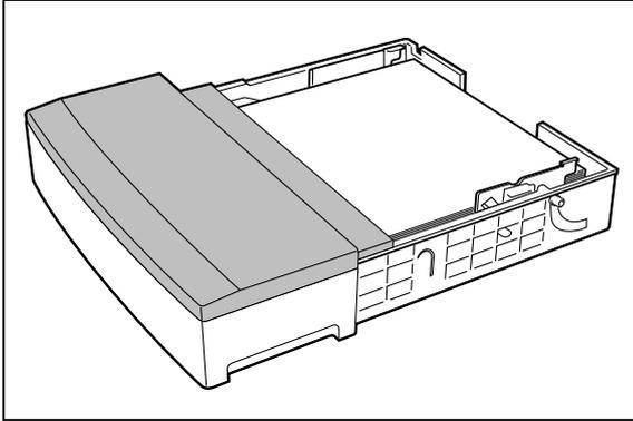
9. Insert the cassette all the way into the printer. Make sure the cassette is properly seated.
