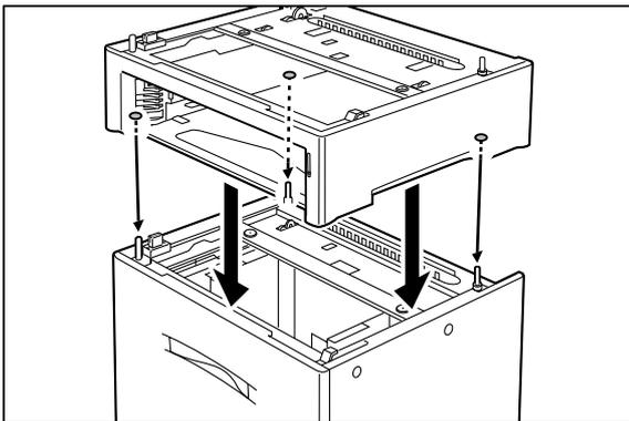
7. Insert the two supplied screws into the holes on the bottom of the printer to secure the HCF unit as well as the paper feeder.
