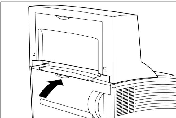
11. Insert the stub on the paper output tray into the hole of the HCS unit to secure the HCS unit.
