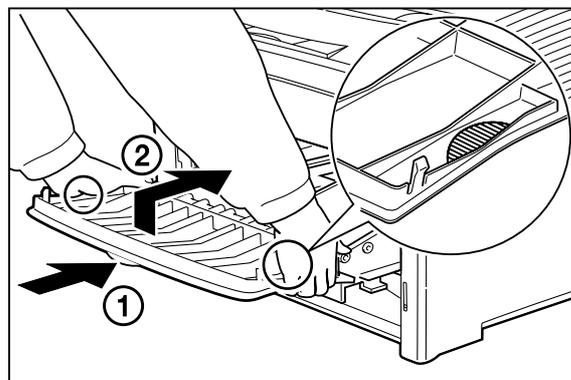
14. Hold the EP cartridge as shown. Then, ① insert the projecting parts on the cartridge into the guide channels of the printer, and ② lower the cartridge into the printer.
