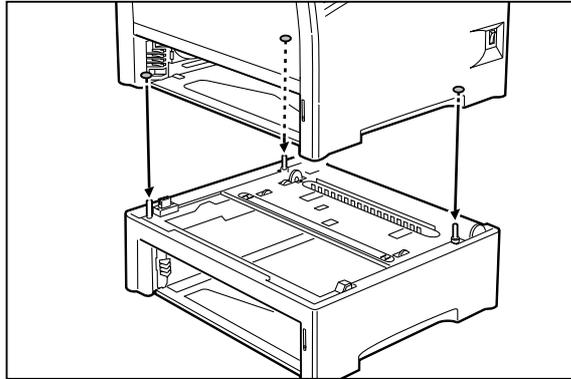
**Important:** Be sure to lower the printer gently, lowering it too fast onto the paper feeders may damage the components inside the printer.
