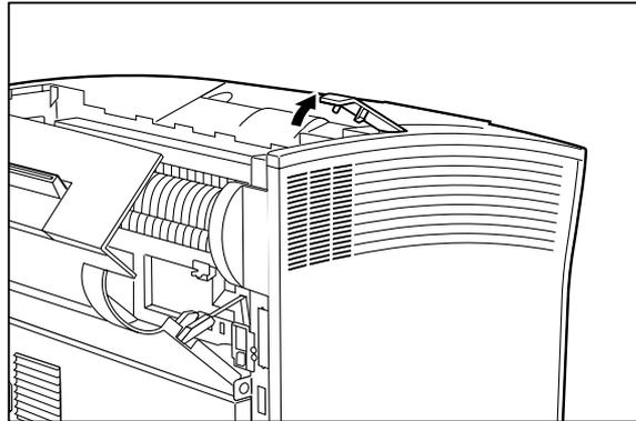
6. Install the attachment of the HCS unit to the rear cover.
