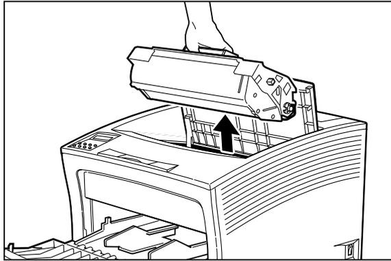
12. Check the area where the EP cartridge was located, and remove any jammed paper.
