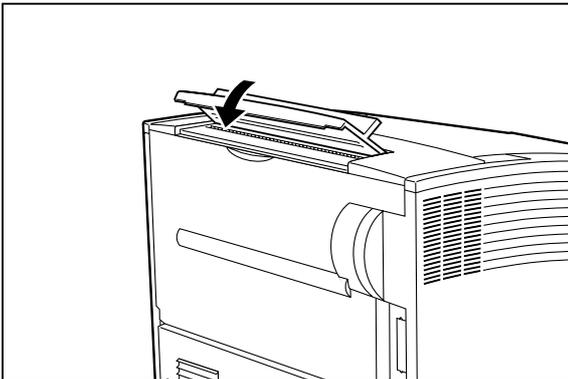
4. Pull on the recessed area on the upper middle part of the rear side of the printer, to open the cover.
