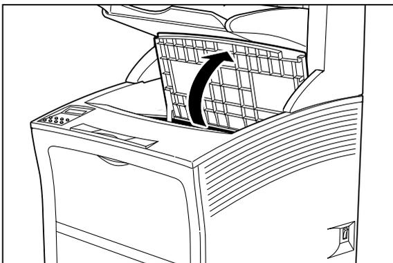
2. Pull on the recessed area on the rear cover of the HCS unit to open the cover, as shown.
