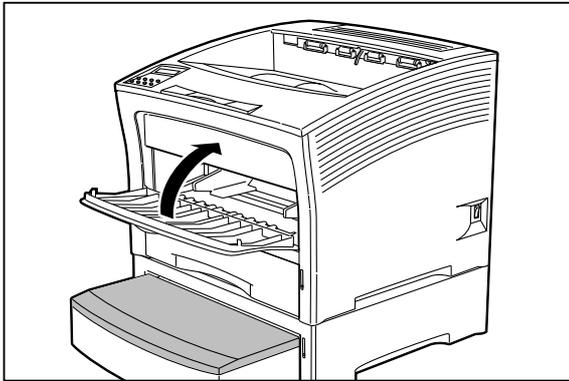
4. Gently lift the cassette up and remove it from the printer.
