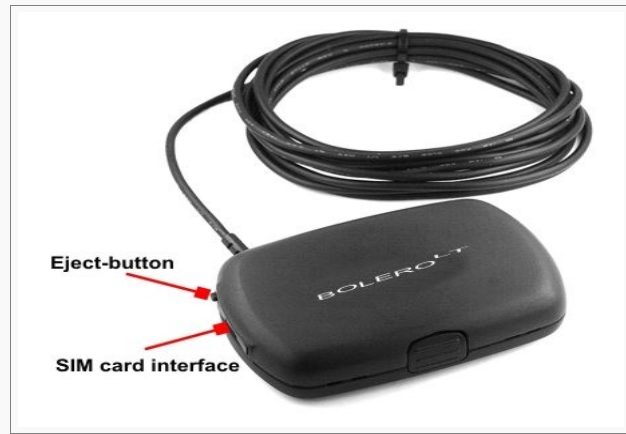
Figure 13: View of the SIM card interface
