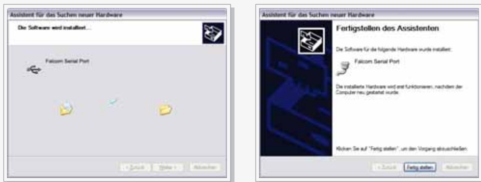
Figure 20: Installing the USB drivers.
