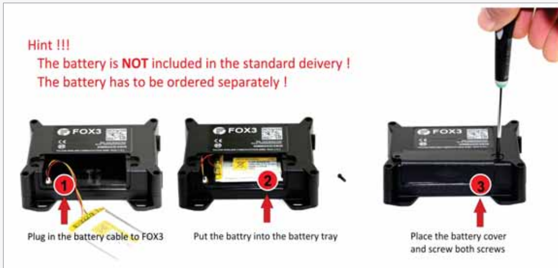
Figure 14.1: Connecting the battery to the FOX3/-3G/-4G devices
