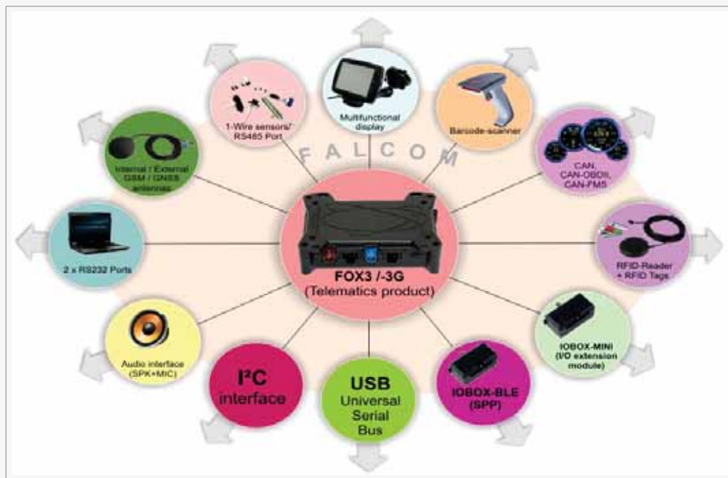
Figure 1: FOX3/-3G/-4G networking and interfaces to peripheral devices.
