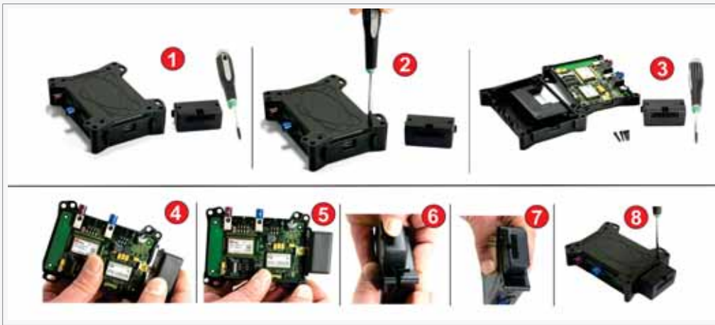
Figure 22: Mounting IOBOX-MINI or IOBOX-CAN to the FOX3/-3G/-4G devices.
