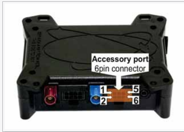
Figure 12: Pin assignments of 6-pin (2x3) connector (Type: MOLEX-43045-06-MICRO FIT)
