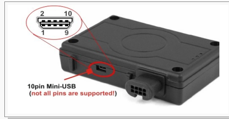
Figure 16: Pin assignments of the 10pin mini-USB (FOX-IN/EN-US).
