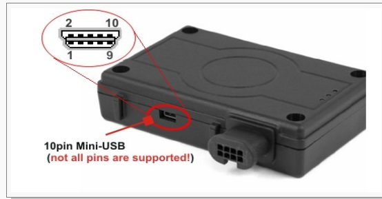
Figure 14: Pin assignments of the 10pin mini-USB (FOX-IN/EN-AU).
