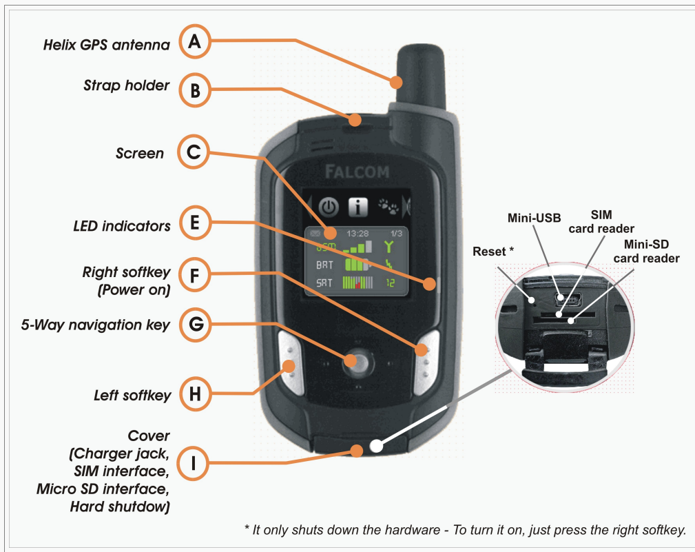
Figure 2: Parts of the MAMBO2
