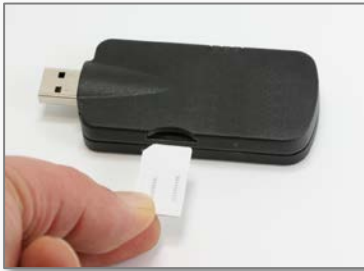
Figure 5.a: Insert the SIM Card.
