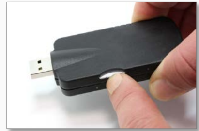
Figure 5.c: To remove the SIM, press the edge of card using your finger nail or a pointed object.
