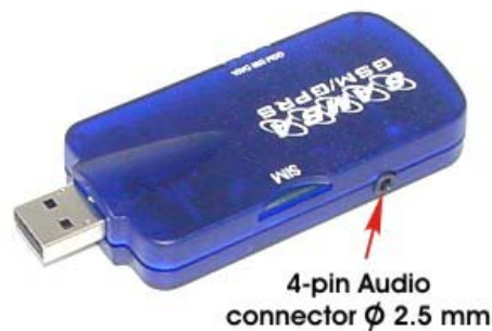
Figure 4: Audio interface pin-out (interface B)
