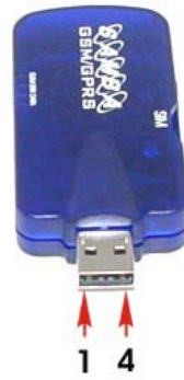
Figure 3: Mini-USB pin-out (interface A)
