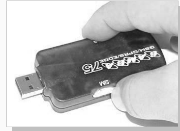
Figure 6: Push it forward into the SIM-Card reader.
