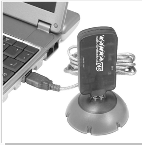
Figure 7: Connect USB connector of SAMBA 75 to the USB serial port of PC. (Note that, the SAMBA-USB-Kit is not a part of modem SAMBA 75).
