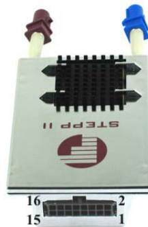
Figure 4: View of the 16-pin Molex 43045-1609 connector pin assignments
