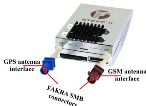
Figure 13: View of the GSM/GPS antenna cable.
