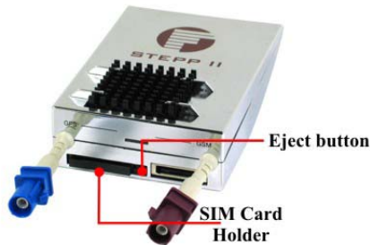
Figure 12: View of the SIM card interface
