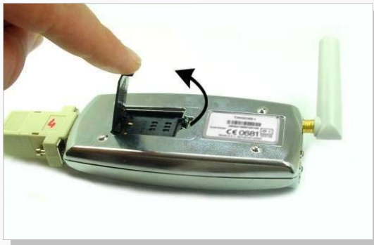
Figure 9: Open the cover cap.
