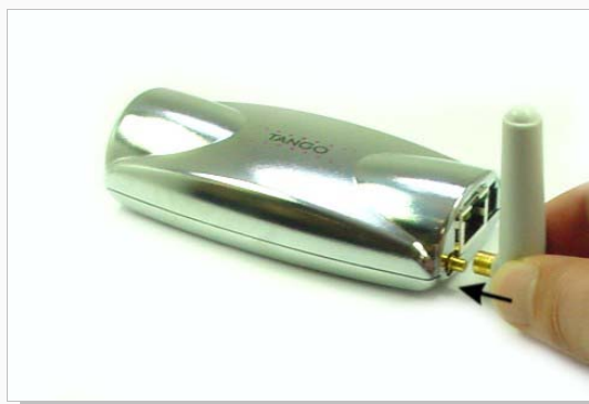
Figure 8: Connect the GSM antenna
