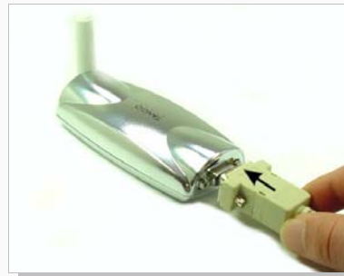
Figure 13.b: Connect 9-pin serial to modem.
