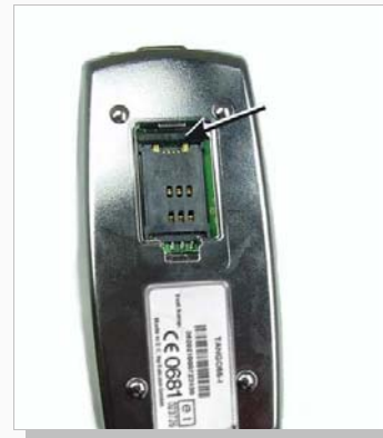
Figure 10: Push the inscription "PUSH ▲ OPEN" to open the SIM card holder.
