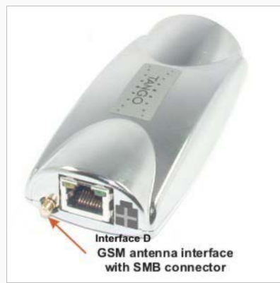
Figure 5.a: TANGO55/56 modem with SMB antenna connector
