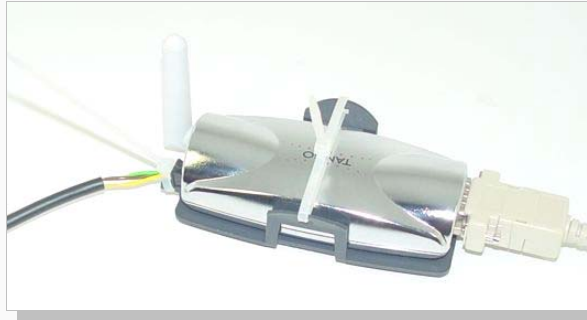
Figure 12.a Place the modem on the cradle and firmly fixed.
