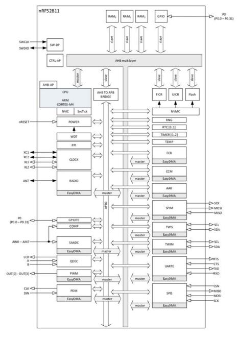
The following is a block diagram of Nordic nRF52811 Bluetooth Low Energy (BLE) SoC.
