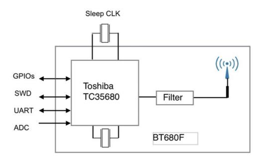
signal. Printed antenna is integrated. Co-existence connection with WiFi is provided.
