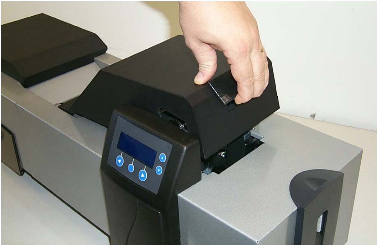
Display A – Loading the Print Ribbon (lift up cover)
