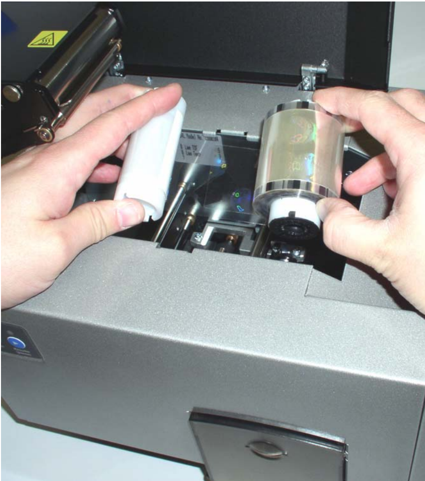
Display A – Loading the overlamine (supply spool)
