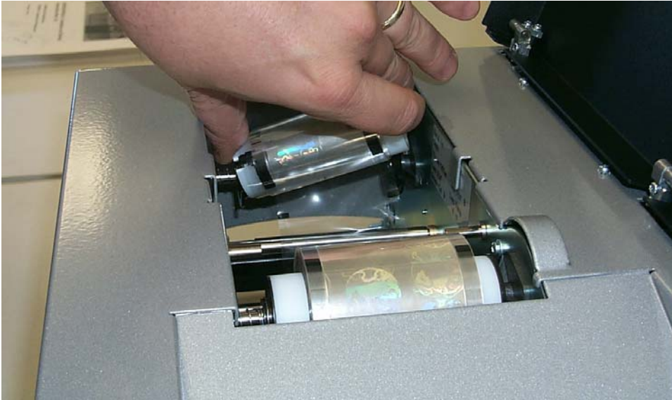
Display B – Loading the overlamine (take-up spool)
