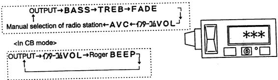
2) By pressing the buttons ② and ③, the setting can be changed.
