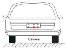
X The ordinary camera can be installed in any water-proof position needed.
