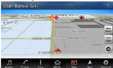
The 3D map is a map screen using a viewing position above the vehicle
