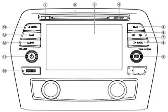
[♠]Eject button: Short press it to eject the disc inside the unit.
