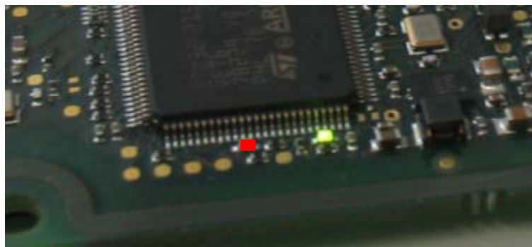
Figure 8: Position of the green and red LED
