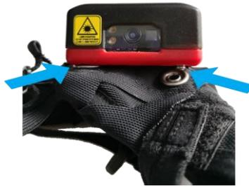
3. Close the lug with the Velcro strip to secure the scanner unit in place.
