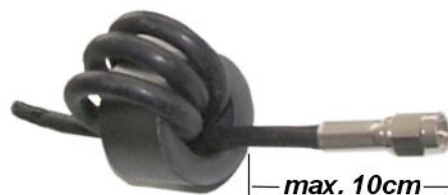
Figure 3: Assembly of the torrid core at the coaxial cable
