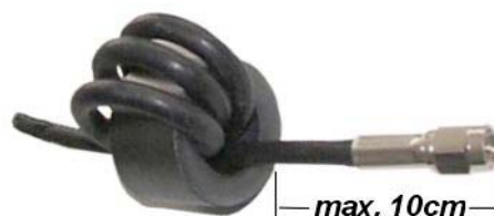
Fig. 3-3: Antenna line with EMC ring cores
