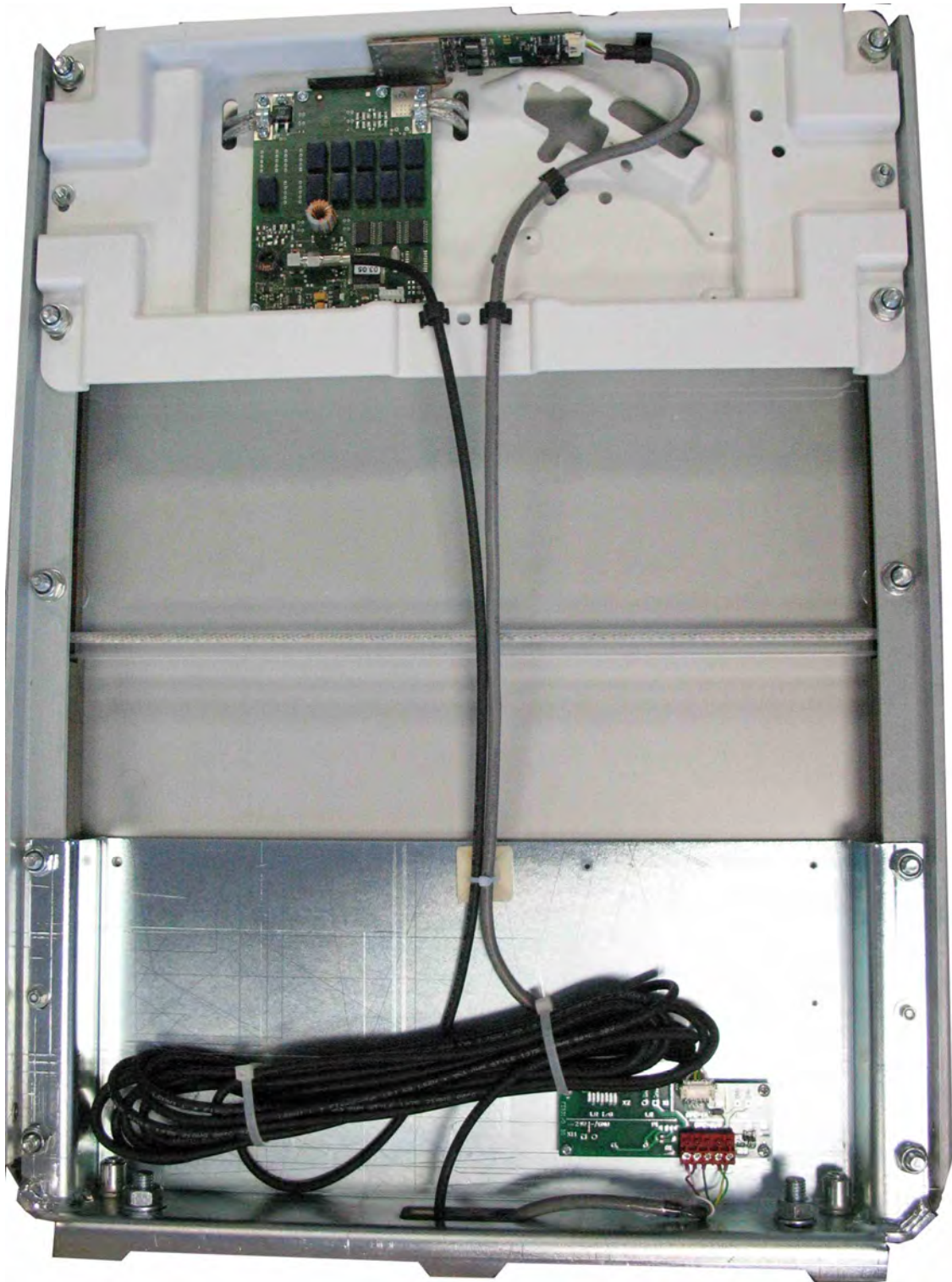
Fig. 17: Unused coaxial cables are tied in antenna Type B
