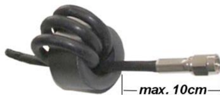
Figure 10: Antenna cable with EMV ferrite core
