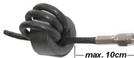
Figure 15: Assembly of the toroidal core at the coaxial cable
