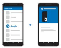
Tap your registered ePass FIDO® Security Key to the mobile device's NFC sensor to complete the authentication;
