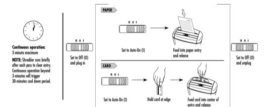
Safety Lock prevents accidental operation. 🔓 To set, wait for shredding to stop, set control switch to Off (0) position, then slide black button down.
