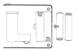
Slide off the battery cover from the back of the MT-30, pop the batteries out, replace with new ones and slide the cover back until it locks. Please pay attention to the polarity.
