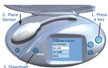
After you have cleaned and dried a key your Sensor, place it on the Reader with the fins neatly aligned in the Sensor well and press the (½) (Download) key.
