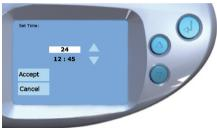
Using the up ▲ and down ▼ keys, select whether you want to use 24 hour or 12 hour clock. For example 23:00 or 11.00 pm, then press Confirm ←
