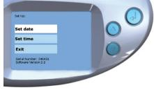
Using the up ▲ and down ▼ keys on the Main menu - highlight the Set Up option, then press Confirm
