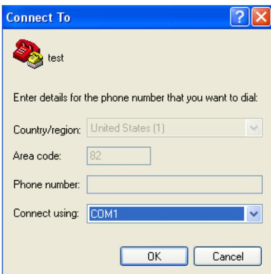
Select each blank as below “Bit/sec: 115200, data Bit: 8, Parity: None, Stop Bit: 1, Flow Control: None”, and click the OK button. Hyper Terminal is executed.
