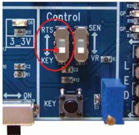
< Figure 7-1-4-(1)-① KEY / RTS selection switch – Select KEY >
