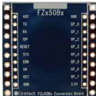
< Figure 7-1-12-⑧ 2.54mm(100mil) A Convertible Board >
