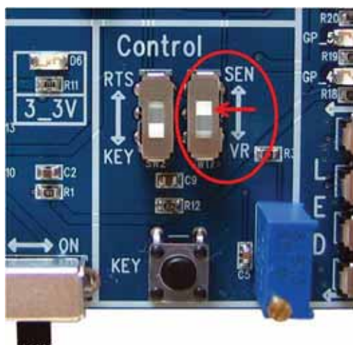
< Figure 7-1-4-(2)-② VR / SEN selection switch –Select SEN >
