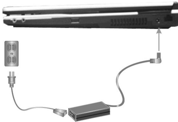
3. Plug the connector of the AC adapter to the DC-IN port found at the left side of the computer.
