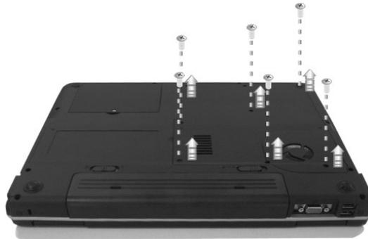
3. Remove the screws and open the DIMM cover by your finger.
