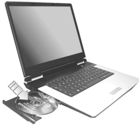
3. To remove the disc, press on the center spindle and pull up the disc from the side until the disc snaps out of the spindle lock.
