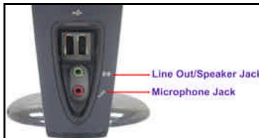
Figure 1-7. Connecting Audio devices via Line-out or Microphone Jack.
