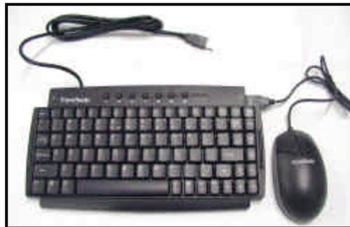
Figure 1-5. Connecting a USB Mouse via USB Keyboard
