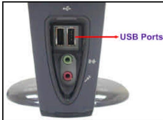
Figure 1-8. Connecting USB devices via USB Connector
