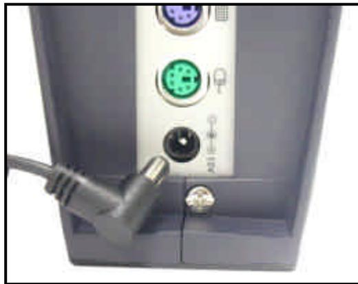
Figure 1-10. Connecting to the Power Adapter
