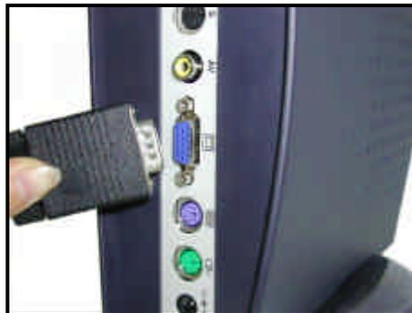
Figure 1-3. Connecting a monitor via VGA Connector
