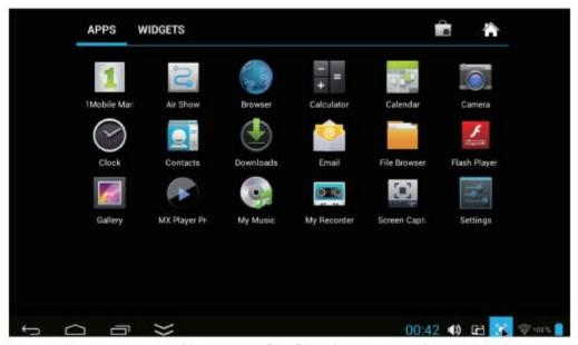
Press on the screen and move Left of Right (Up or down) to show more selections. Press the corresponding button you need to set. The sub-setting menu will appear on the screen, follow on screen instructions.
