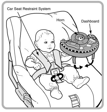
Before attaching the dashboard to your car seat's restraint system, check to be sure the car seat restraint system is securing your child properly. Check all restraint system belts (shoulder, lap, crotch, etc.) by pulling on them. The straps should not pull more than one inch (two fingers) away from your child.
