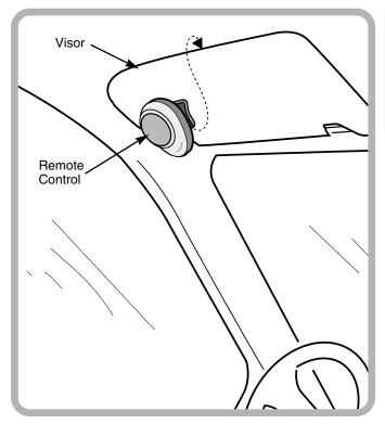
• Attach the remote control clip to the top of the vehicle visor, as shown.
