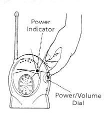
Place receiver in room in which you intend to use it. Rotate power/volume dial to turn power on. Power indicator lights. Adjust receiver location.
