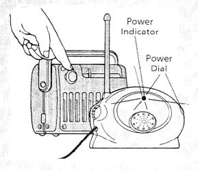
Place transmitter in room in which you intend to use it. Rotate transmitter power dial to turn power on. Power indicator lights. Turn on a radio.
