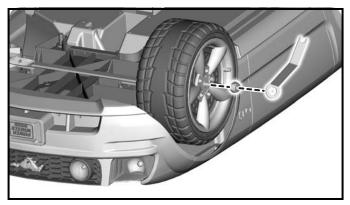
Fit a <sup>3</sup>/<sub>8</sub>"-16 lock nut, *rounded side out*, onto the front axle.
