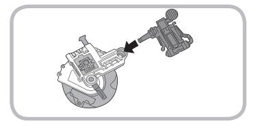
• "Snap" the peg on the backpack into the socket in the tool arm.
