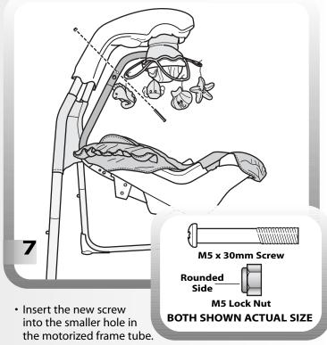
**Hint:** You may need to tap the screw with a hammer or twist the screw to completely insert it through the hole.
