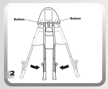
Press the buttons on the back of the motorized frame while pushing the legs inward.
