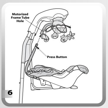
• Press the button on the seat tube and slide the seat tube into the motorized frame tube. Make sure the button on the seat tube "snaps" into the larger hole in the motorized frame tube.
