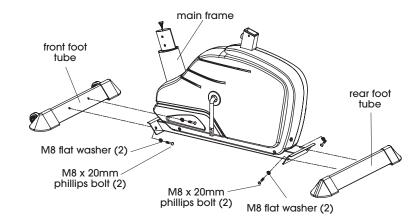
Figure 1 - Install Foot Tubes
