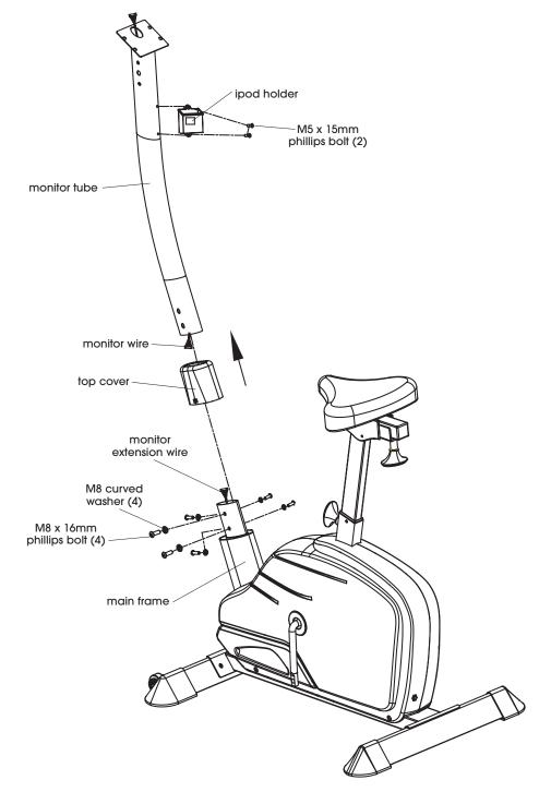
Figure 3 - Install Monitor Tube
