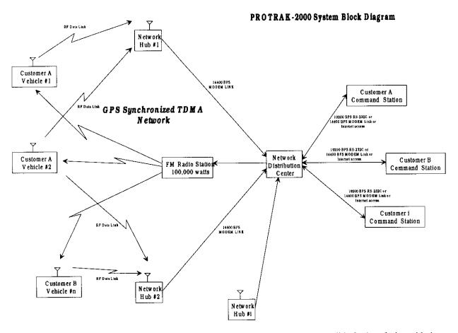
The brain of system is the Network Distribution Center (NDC). The NDC is responsible for interfacing with the customers via a modem on a Public Switched Telephone Network (PSTN) line or the internet, and interfacing with the customer vehicles through Network Hubs and an FM Radio Station(s).
