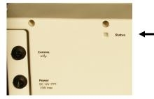
A multi-color LED status indicator is located on the rear panel of the sensor.
