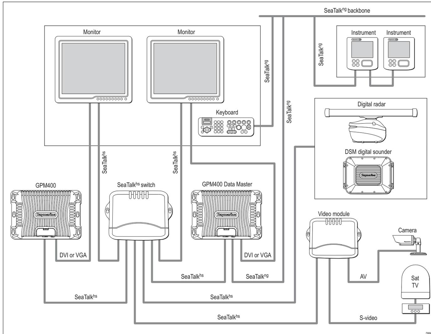
**Note:** Each display at a Nav station must be connected to a different GPM400. Displays sharing a GPM will both display identical information.
