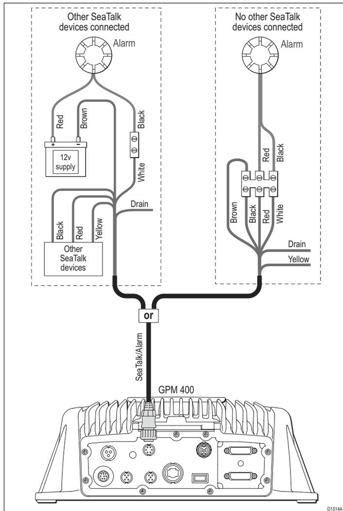
The alarm output and SeaTalk are combined into a single connector. This includes a 12 V fused power supply.
