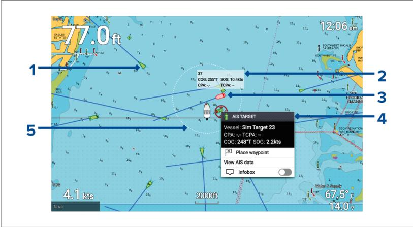
1. **AIS target icon** — Example of an AIS target icon.
