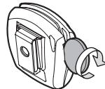
2. Taking care not to disturb other internal components, insert the supplied CR2 3V battery
