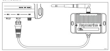
The Wireless hub is required to allow connection of wireless handset stations to the Ray90 / Ray91 base station.
