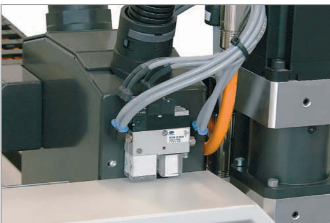
Central vacuum generation by compact ejectors SCPM
