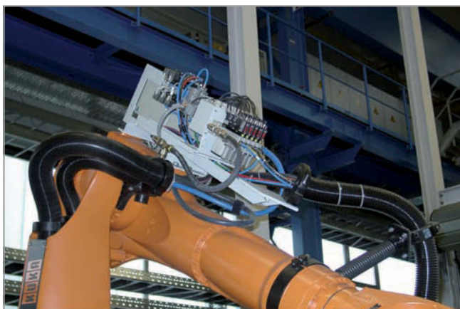
Central vacuum generation by compact ejectors SMP
