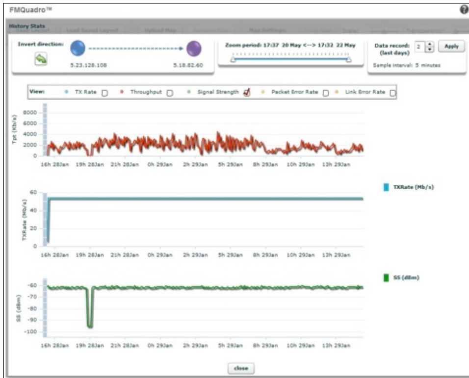
Figure 7.13: FMQuadro, Last 48 Hours Link information
