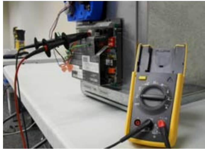
The technician can leave the 233 meter connected to the controller while he carries the detachable display to a computer workstation.
