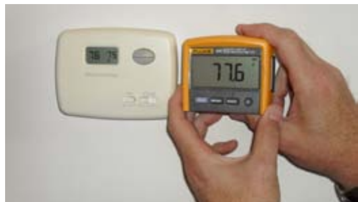
A technician can compare the results on the 233's detachable display to the reading on a remote thermostat.
