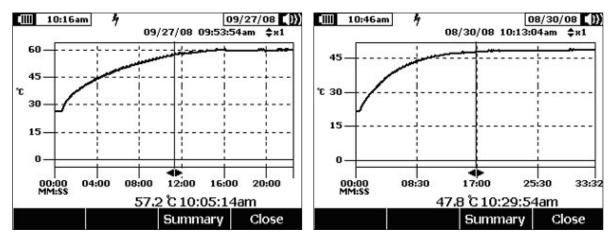
Figure 1. Left Screen Shot shows an amplifier that is running too hot. Right Screen Shot shows an amplifier running at normal temperature.
