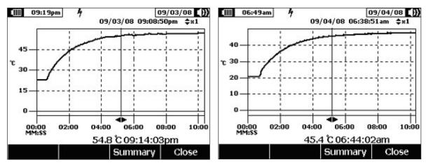
Figure 4. Screen shots showing temperature of 3-terminal regulator IC before capacitor replacement, left, and after capacitor replacement, right.
