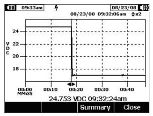
Figure 2. Screen shot showing the controller IC supply voltage as the supply is being turned on. Before the supply is enabled, the voltage is about 24.75 V and drops to approximately 17 V.
